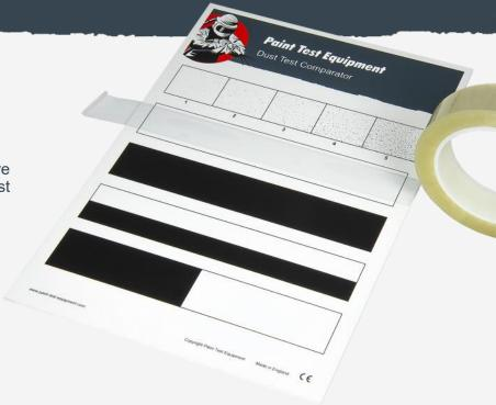
Remove a piece of Tape about 250mm long. Holding the Tape only at the ends, press approximately 200mm of the freshly exposed Tape onto the blast-cleaned surface.
