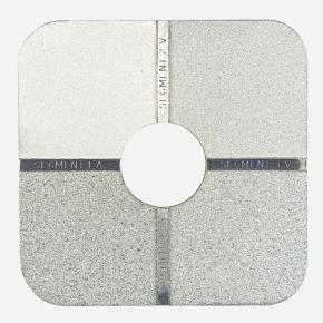
When steel has been blast-cleaned, the surface consists of random irregularities with peaks and valleys that are not easily characterised. Because of this random nature, experts have recommended that the profile should be identified as either angular (where grit abrasives have been used) or dimpled (where shot abrasives have been used) and that they should be graded as fine, medium or coarse with each grade being defined by limits specified in ISO 8503.
