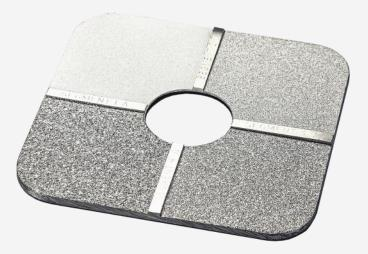
Place the selected Comparator against an area of the test surface. Compare in turn the test surface with the four segments of the Comparator, using the Illuminated Magnifier if necessary. If the Illuminated Magnifier is used, place it so that the test surface is viewed simultaneously with a segment of the Comparator.
