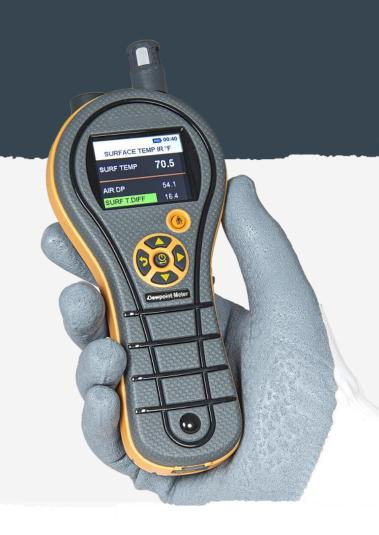
The steel surface temperature generally should be at least 3°C above the dew point when paints are applied. Below this temperature the Dewpoint Meter will sound an alarm and the display colour will change to warn you that the surface conditions are not suitable too paint.
