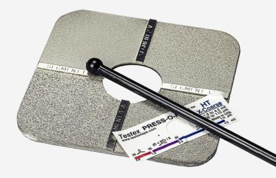
Remove a single piece of Replica Tape from its release paper. The replica material is the square, white plastic film in the centre. A bulls eye circle of paper should remain behind on the release paper (this is not used in the measurement).
