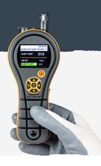
The steel surface temperature generally should be at least 3°C above the dew point when paints are applied. Below this temperature the Dewpoint Meter will sound an alarm and the display colour will change to warn you that the surface conditions are not suitable too paint.
