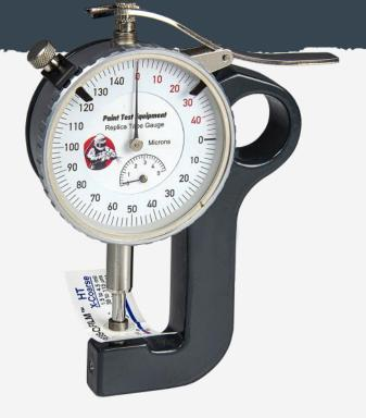
The Replica Tape Gauge is used to measure the Testex Replica Tape replica and determine the average maximum peak-to-valley height of the blasted profile.
