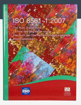
The Book identifies four levels (designated as Rust Grades) of mill scale and rust that are commonly found on surfaces of uncoated erected steel and steel held in stock. It also identifies certain degrees of visual Cleanliness (designated as Preparation Grades) after surface preparation of uncoated steel surfaces and of steel surfaces after overall removal of any previous coating.
